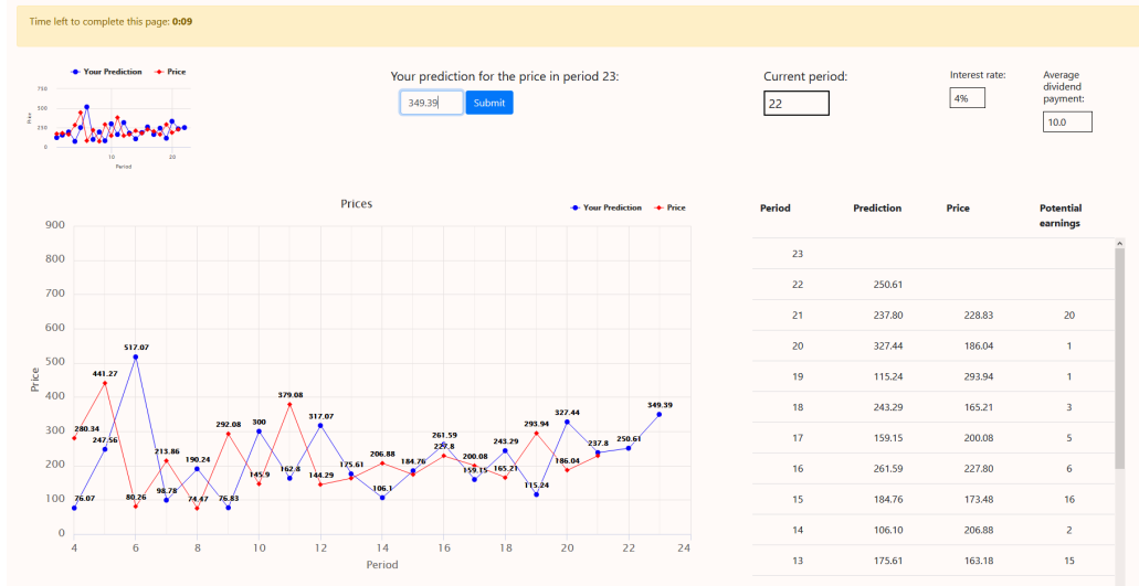
Figure 1: An example of the computer screen. The graph shows past predictions (blue) and past prices (red). The table provides the same information, and in addition, the “Potential earnings”, that is, the points for each period if that period is selected for payment (using Eq. (5)). A prediction can either be typed into the box in the top middle of the screen or indicated by clicking the mouse button on the graph in the lower part. In the H and L treatments, the prediction is submitted automatically as the decision time runs out. To submit the prediction in the HS treatment, participants must either press the ‘Enter’ button on the keyboard or click the blue ‘Submit’ button on the top of the screen.
